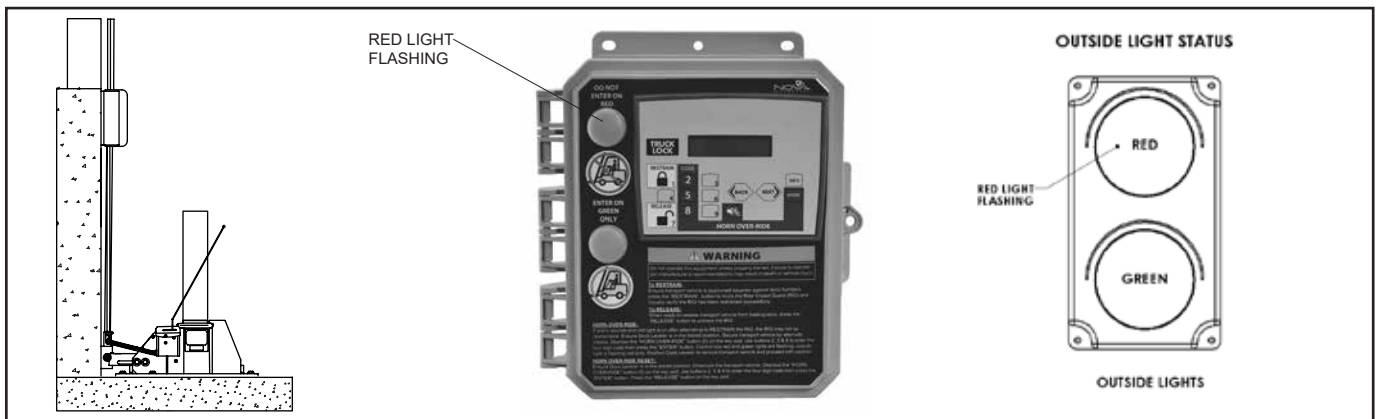
Figure 5-5-13 RESTRAIN position, horn sounding
