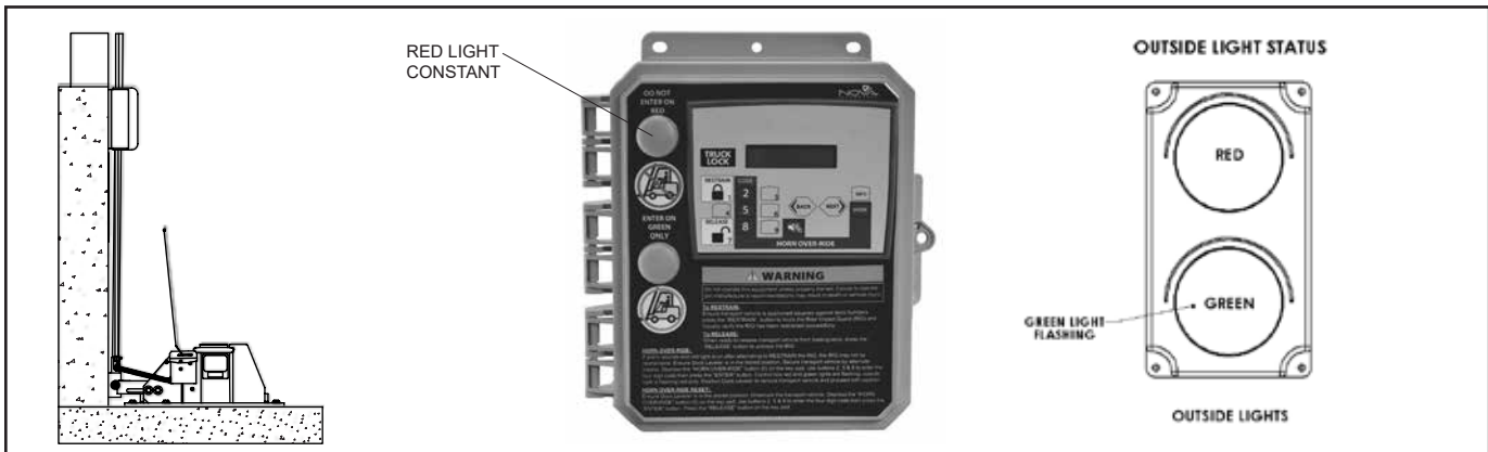
Figure 5-5-16 Restraint released, RIG sensor activated
